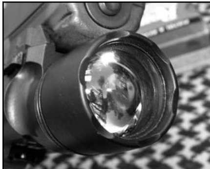
The SureFire X200 utilizes a specially designed lens to focus the LED beam. The lens is recessed for better protection.
